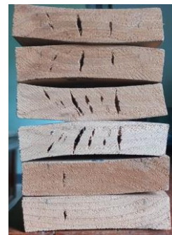
Figure 4. Deformation and honeycombing in 30 years old plantation teak
