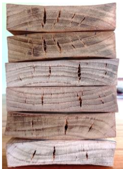
Figure 3. Deformation and honeycombing in 34 years old plantation teak
