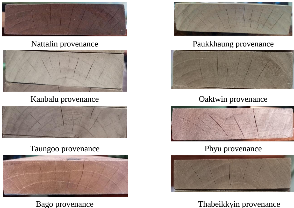
Fig 5. End checks in 15 years old plantation teak from provenance trial
