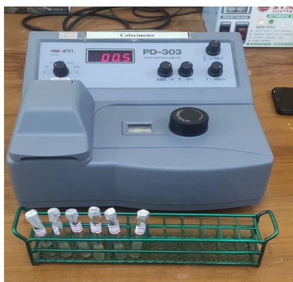
Figure 22. Absorbance reading for broth cultures dilution to obtain the OD 600 at 0.08 to 0.1
