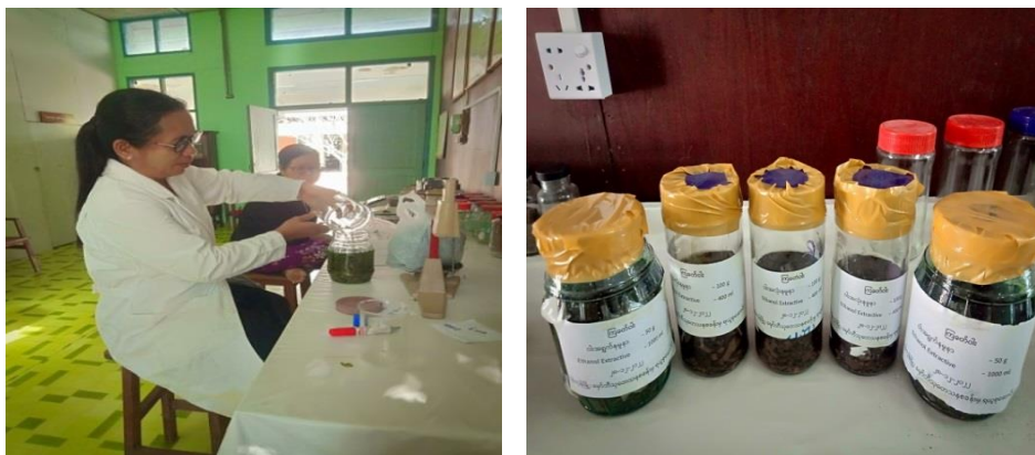
Figure 5. Making Extracting the Burst Bamboo Stem and Leaf with Ethanol
