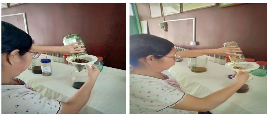
Figure 6. Filtering the Extraction Mixture Solution to Get Extract Liquid
