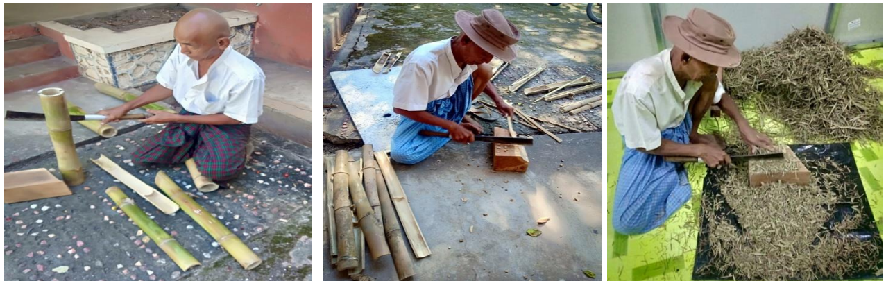
Figure 3. Sample Preparing; Cut the Dried Bamboo Stem and Leaf
