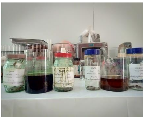
Figure 7. Drying the Filtered Extract Fluid at Room Temperature about 3 Month
