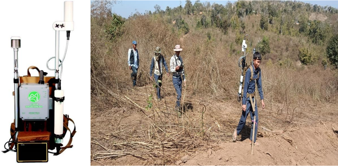
Figure 4 Magnetometer G-864 SX (left) and magnetic surveying in the field (right).
