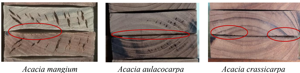
Figure 4. Honeycombing and deformation in three Acacia species
