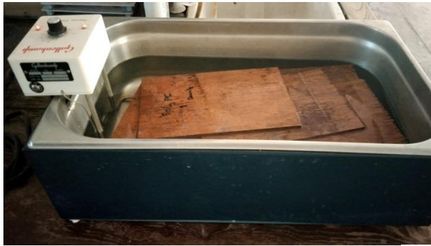
Fig 17. BWR testing of PF samples
