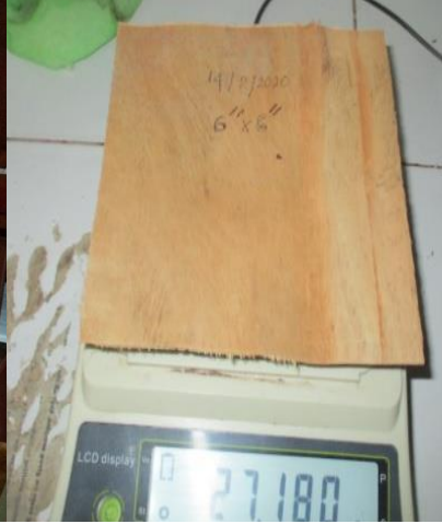
Fig 8. Determination of Moisture Content of Veneer Thickness
