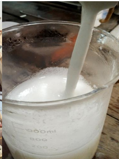
Preparation of UF resin
