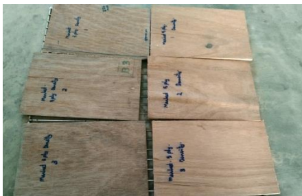
Fig 15. Sample Boards for MC and Density
