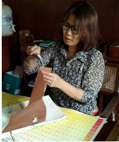
Fig 7. Measurement of Veneer Thickness
