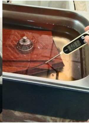
Fig 18. MR testing of UF bonded plywood
