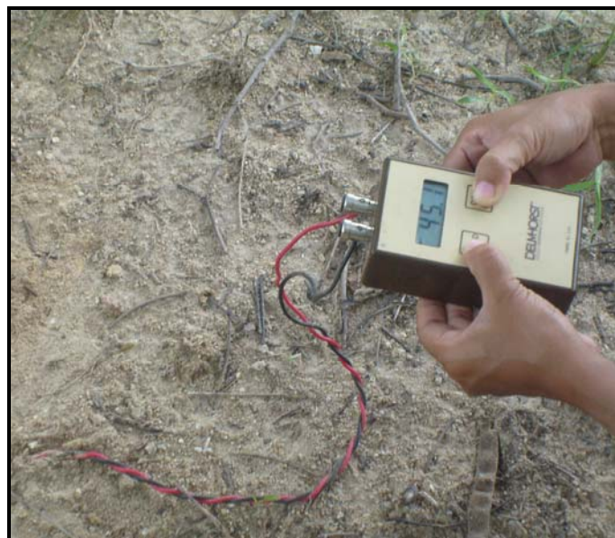
Figure 4. Measuring of soil water potential with Delmhort soil moisture meter Model KS-D1.
