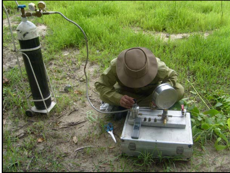
Figure 3. Measuring plant water potential with the Scholander apparatus in the field.
