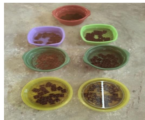
Figure 16: Photo showing Water absorption testing of wood sample
