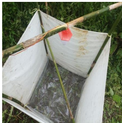
Figure 4: Setting light trap (up sight and lateral sight)
