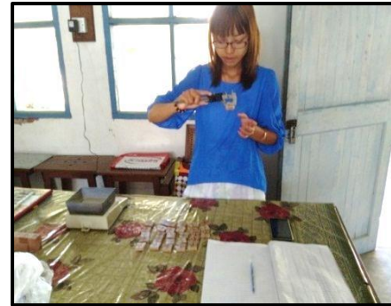
Figure 6: Photo showing measurement of dimensions of wood sample
