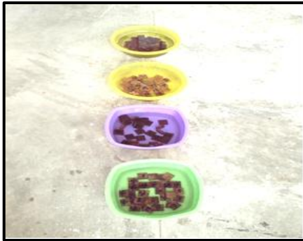
Figure 5: Photo showing water absorption testing of wood sample
