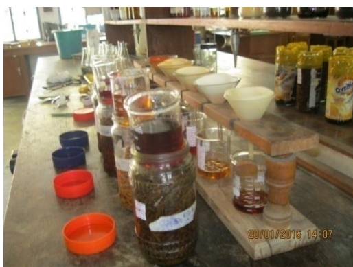
Filtering the sample extract
