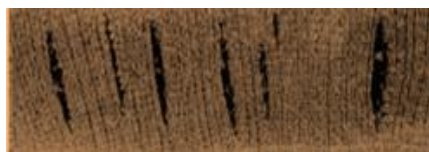
Figure 3. Honeycomb (internal checks) in the cross section of wood
