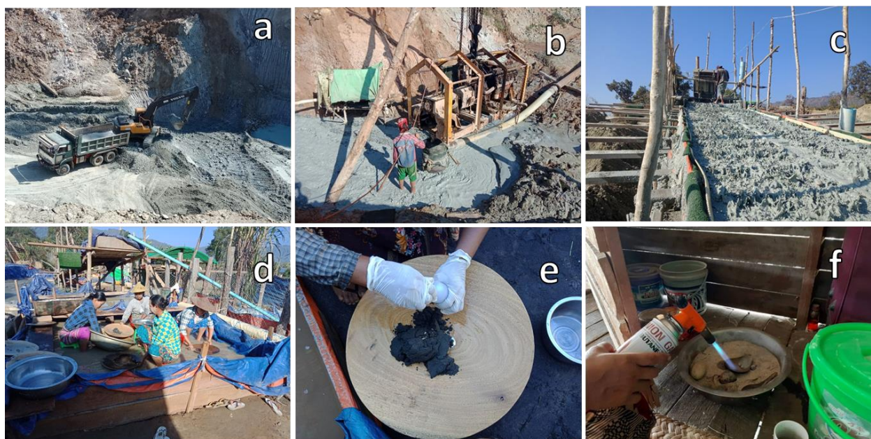
Figure 2. Placer small-scale gold mining in Banmauk Township: (a) Removing surface soil by using backhoe and truck. (b) Ore processing by adding water. (c) Sluicing through wooden sluice. (d) Panning by using wooden pan. (e) Recovering gold particles by adding. January 25, 2019.
