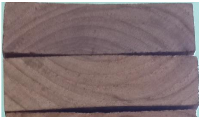
Fig(4) Deformation in 37- and 32-year-old plantation teak
