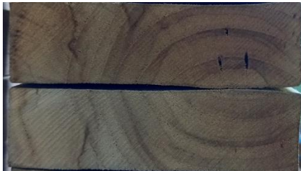
Fig(5) Deformation and honeycombing in 20-year-old plantation teak
