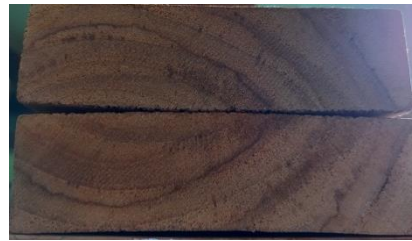
Fig(3) End checks and Deformation in 40-year-old plantation teak
