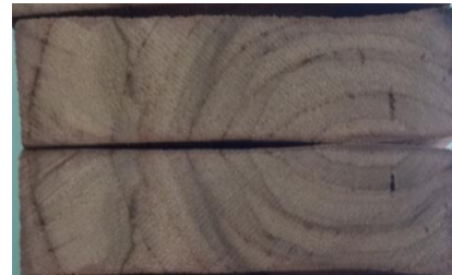
Fig(5) Deformation and honeycombing in 20-year-old plantation teak
