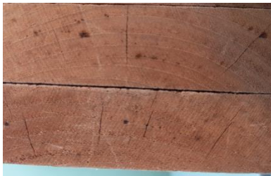
Fig(3) End checks and Deformation in 40-year-old plantation teak
