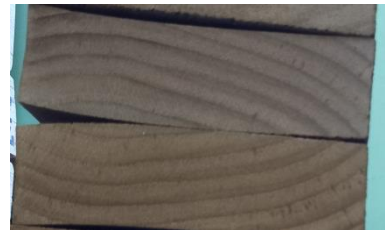
Fig(4) Deformation in 37- and 32-year-old plantation teak
