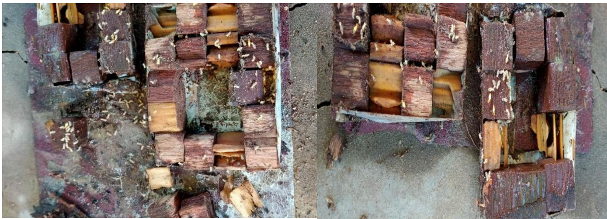
Figure 5.7 Photo show termite attack for untreated wood samples.
