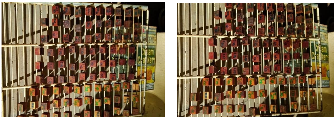
Figure 5.8 Photo show termite attack for Extracted treated wood samples.
