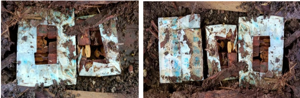
Figure 5.6 Photo show termite attack for untreated wood samples.
