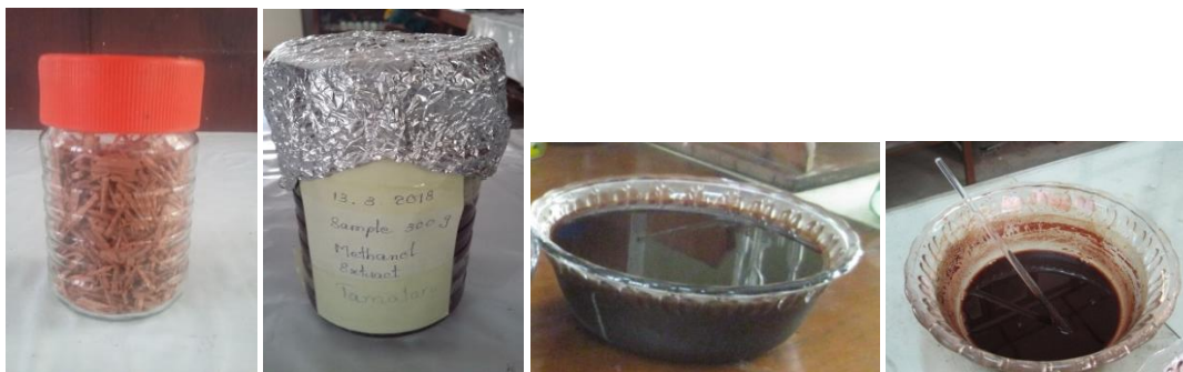
Figure 3.2 150 ml of 0.3 % HCl in Methanol Extraction
