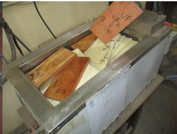
Figure 22. MR testing of UF bonded plywood
