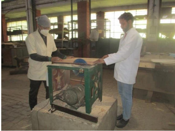
Figure 13. Trimming of plywood
