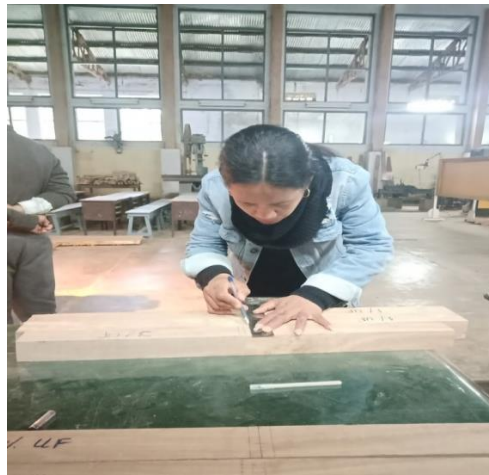
Figure 3.1 After drawing the Centre line to make finger joint
