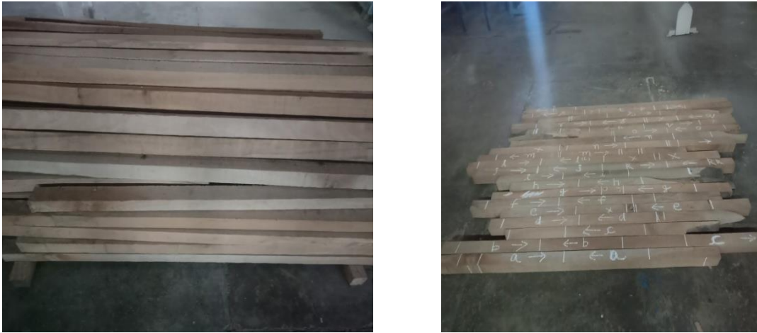
Figure1. Choice of defect, crack and node
