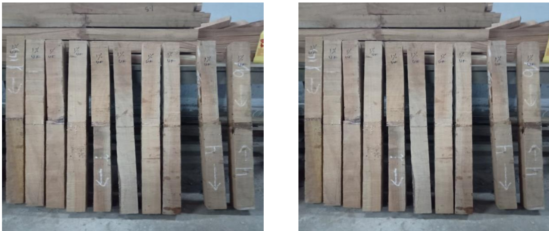
Figure 9. Curing the finger joint at room temperature
