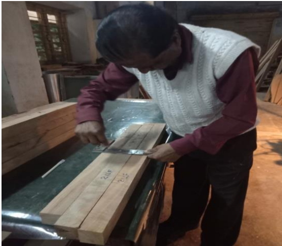
Figure 3.1 After drawing the Centre line to make finger joint
