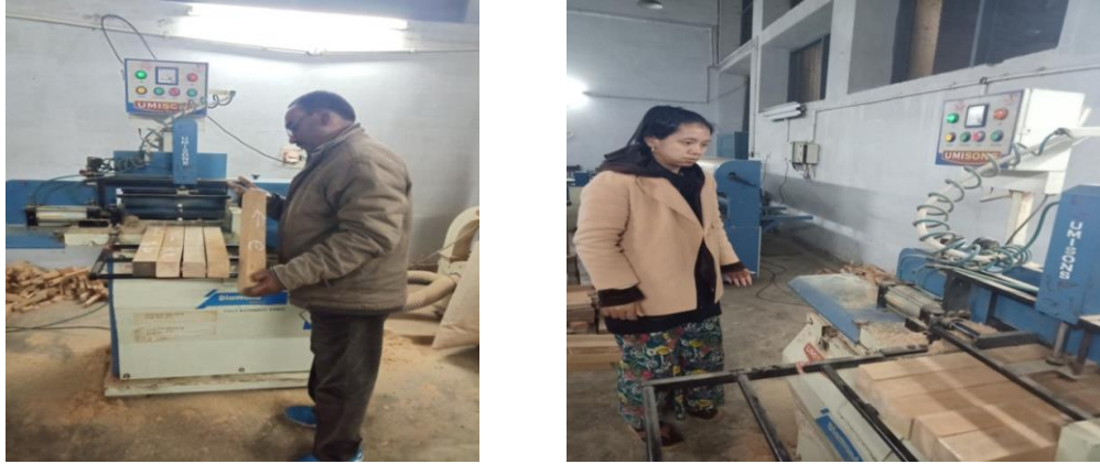
Figure 4. Preparation of finger by commercial finger shaping machine
